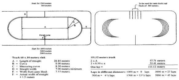
2. The demarcation of the tracks and the turns should be indicated with coloured markings and/or moveable blocks of rubber or other suitable material.
